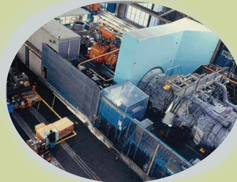
Aerodynamic probe measurements and dynamic pressure measurements in a heavy duty gas turbine to verify the design and off design performance and to provide a data base for the development of a compressor stability monitoring system
